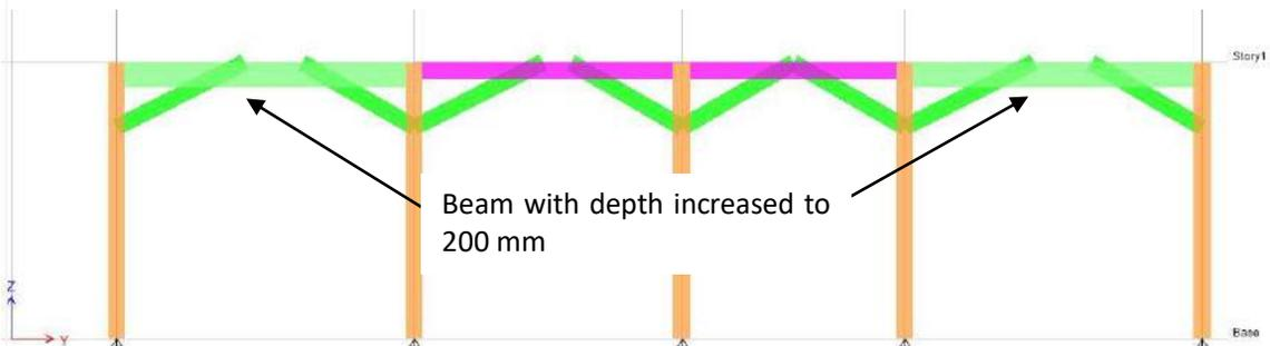
**Figure 6: Beams with depth increased to 200 mm**
