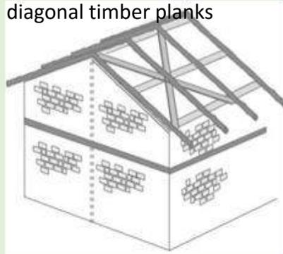
Diagonal steel bracing to roof
