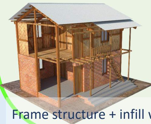
Frame structure + infill wall
