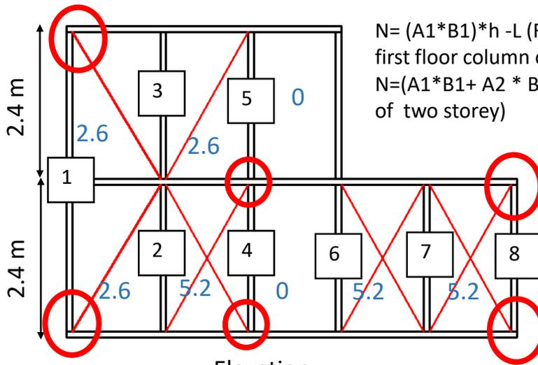
$N = (A1*B1)*h - L$  (For single storey column and first floor column of two storey)
