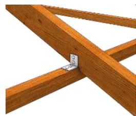
Detail B: Joints of Wooden Truss
