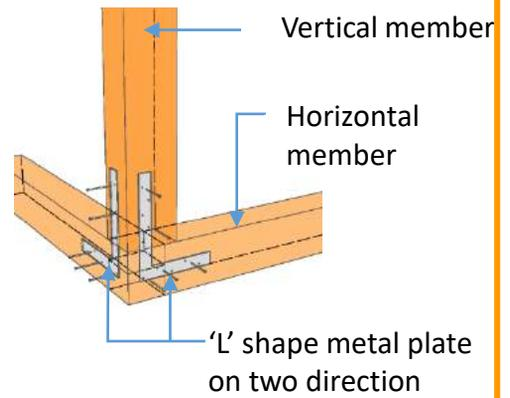
Detail B: Connection horizontal and vertical at middle
