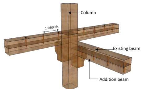
OPTION 2. Connection details of addition of horizontal member through wooden nails
