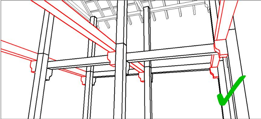
*Note: Add new beams in missing direction with constructability approach (i.e. beam in all direction may be in different level).*
