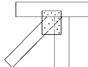
**Note:** Instead of metal plate, three layers of 0.55mm GI sheet can be used.
