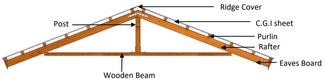
A **timber roof truss** is a structural framework of timbers designed to bridge the space above a room and to provide support for a roof. Trusses usually occur at regular intervals, linked by longitudinal timbers such as purlins.
