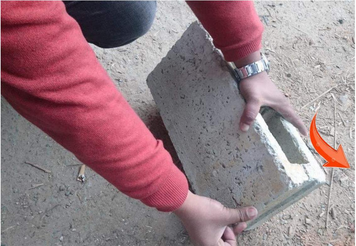
Press the corner of the block. It should not break.
