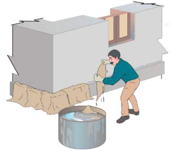
An illustration showing a construction worker in a blue shirt and orange hard hat kneeling on the ground. The worker is applying jute bags to the wall to cure the concrete. The wall has a window opening. The worker is positioned at the base of the wall, where the new horizontal band is being added. A bucket of water is visible on the ground. |
