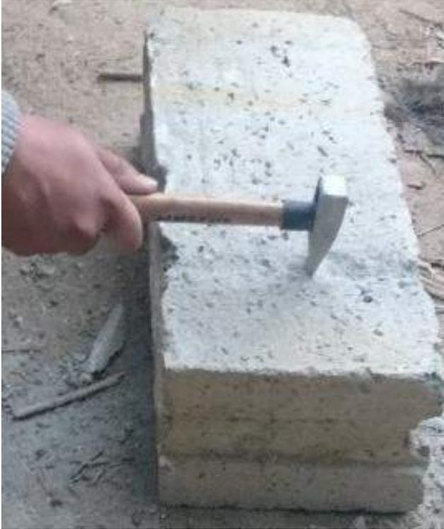
Cut the block with chisel at the centre as shown beside. Block should always break only in two pieces. If it breaks into many pieces, it indicates low strength.
