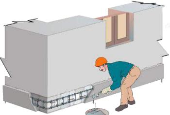
An illustration showing a construction worker in a blue shirt and orange hard hat kneeling on the ground. The worker is applying a layer of micro-concrete to the wall using a trowel. The wall has a window opening. The worker is positioned at the base of the wall, where the new horizontal band is being added.                                    |
